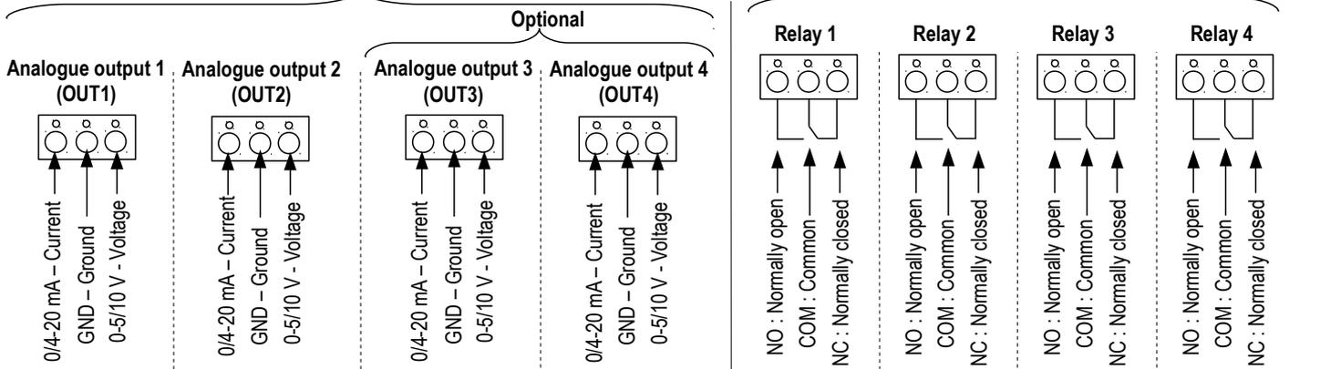
(c) For 24 Vdc/Vac power supply models:
